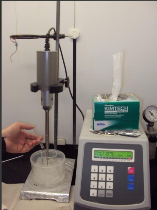
Mixing of continuous and discontinuous phase during sonication
